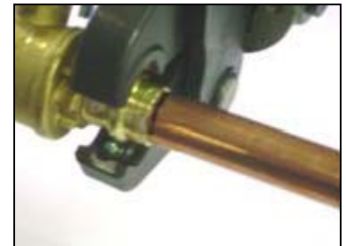
I. After pressing, release the jaws and remove the tool. Do not attempt to adjust the valve on the pipe after pressing.
