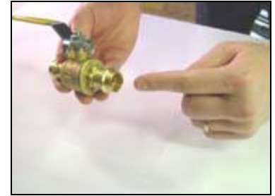
C. Check seal for correct fit. Do not use oils or lubricants. Use only the valve's yellow NBR o-ring seals.
