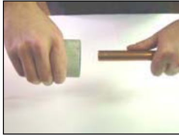
B. De-burr tubing on the inside and outside to prevent cutting of the valve's o-ring seals.
