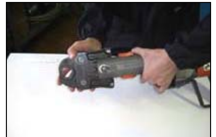
F. Insert the appropriate jaw into the pressing tool and push in holding pin until it locks into place.
